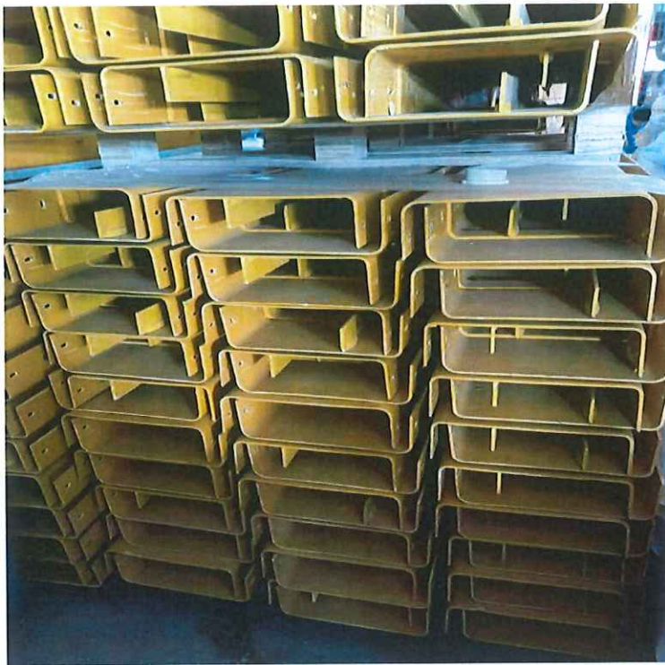
隧道低压线缆防火槽盒
